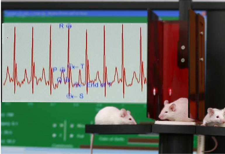
Three conscious mice atop the **ECGenie** instrumentation. The ECG signal is detected passively through the paws of the center subject, as the other two subjects acclimatize to the **ECGenie** recording platform.
